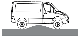
Transfer case ground clearance approx. 360 mm
