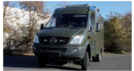
All-wheel drive conversion for special use in desert regions with a lot of diverse off-road equipment
