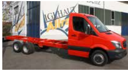
Increase in load capacity up to 7.49 tons by installing a third axle
