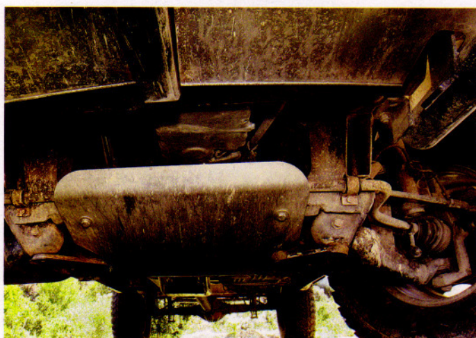
Out of harm's way: Protection plates keep vulnerable components safe. With a 300 mm ground clearance, there is not much work for them to do
